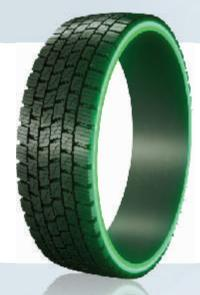
RINGTREAD is the only retreading system that uses splice-less precured rings that adhere perfectly to the casing without a splice, tension or deformation. This means lower fuel consumption and less emissions. The perfect geometry and the use of latest-generation compounds assure higher mileage and better grip under any road condition.
